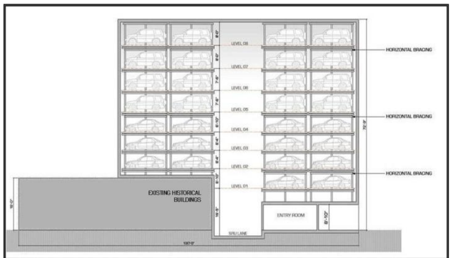
Cross-section of Parking Facility
